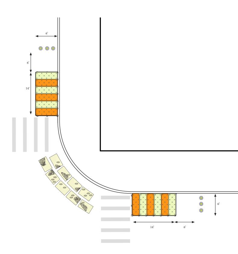
Fig. 04: Curb Extension Plan Diagram
