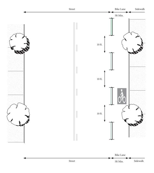
Fig. 03: Separated Bike Lane Plan
