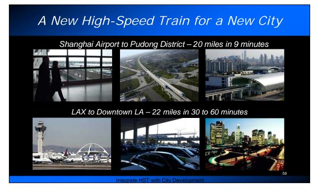
An integral part of Shanghai's growth plan is a new high-speed line connecting Shanghai's Pudong district with a new airport located some 20 miles from the city center. Traveling at a top speed of 271 miles per hour, the high-speed line makes the 20-mile trip in a mere 9 minutes (average speed 133 mph).
