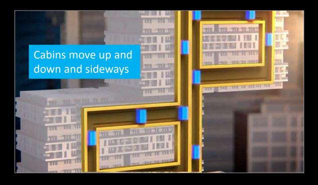
minute away from a passenger stop, travelling 16 feet per second, or about 11 miles per hour. Maglev cabin movers would enable a staggering 40 per cent increase in usable floor area in a multi-story building.
